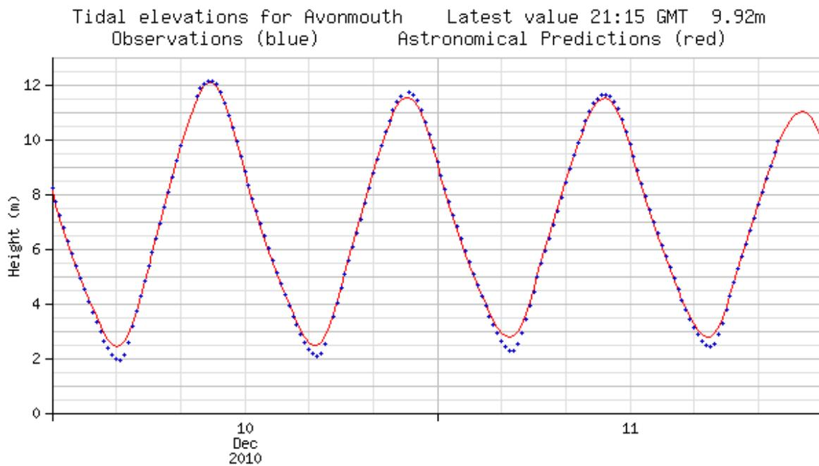
The rise and fall of the tide is at a rate of 25mm per minute in the Bristol Channel/Severn estuary with very limited static periods of high and low water. In the some parts of the Severn estuary levels change at rates of 35mm per minute or higher.
